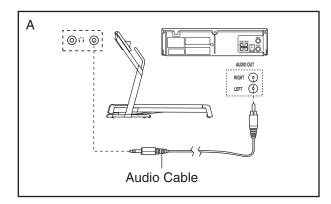
B. Plug one end of a long 3.5 mm to RCA stereo audio cable (available at electronics stores) into the input jack on the console. Plug the other end of the cable into an RCA Y-adapter (available at electronics stores). Next, remove the wire that is currently plugged into the AUDIO OUT jack on your VCR and plug the wire into the unused side of the Y-adapter. Plug the Y-adapter into the AUDIO OUT jack on your VCR.
